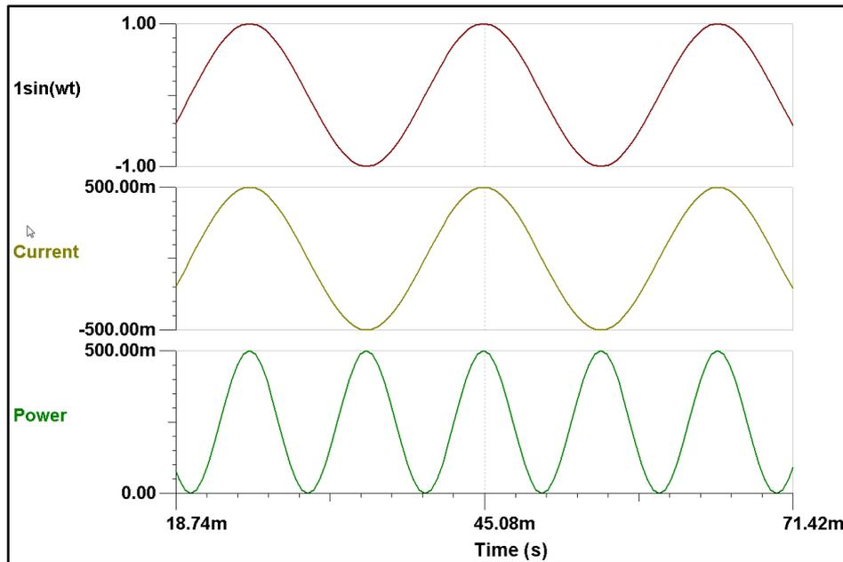
Fig(3) : Voltage current and power dissipation waveforms
