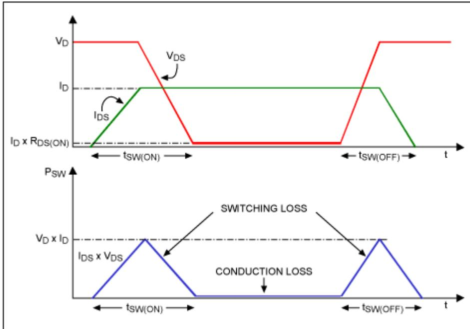
**Fig (4):** Switching losses timing diagram
