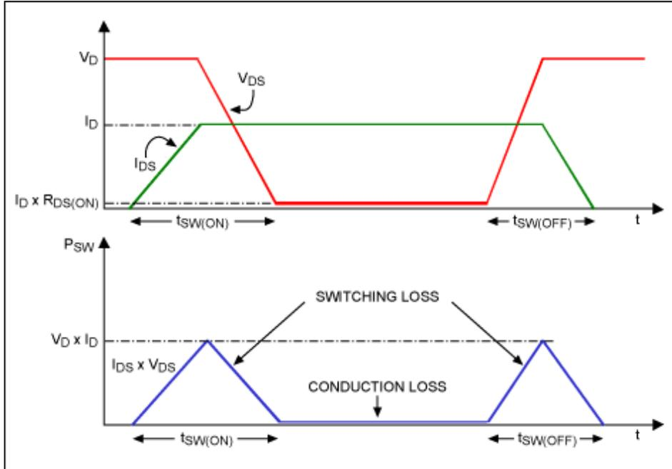
**Fig (4):** Switching losses timing diagram
