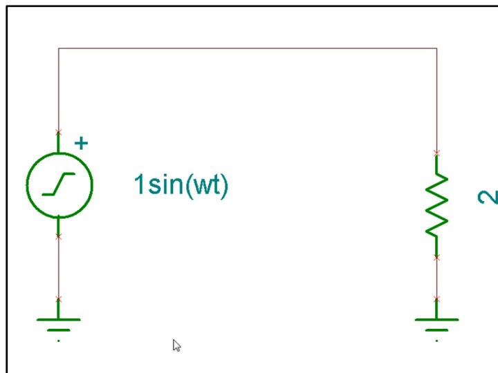
**Fig (2):** Voltage  $V = 1 \sin(\omega t)$  applied across a resistor of value  $2 \Omega$
