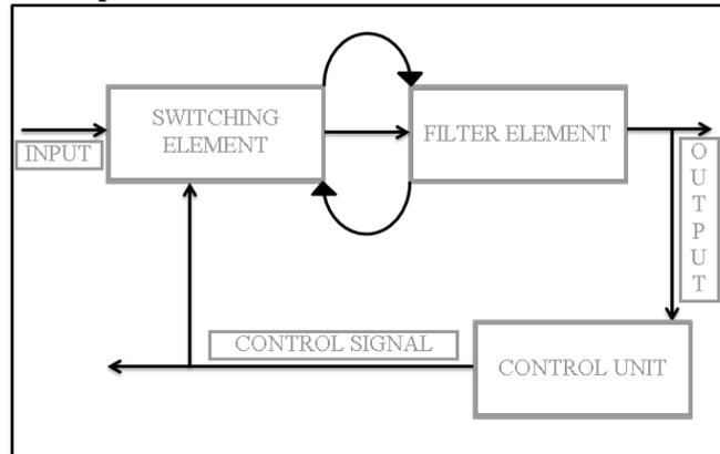
**Fig (1):** General structure of a switch mode power converter
