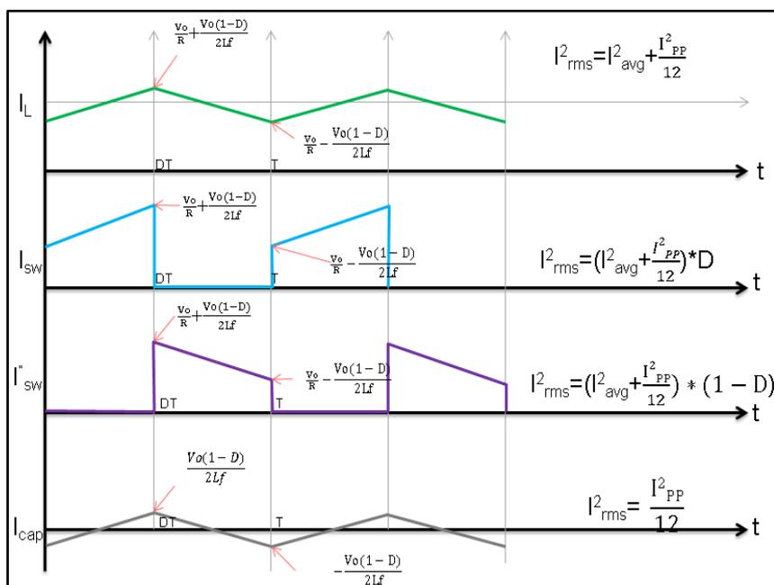
Fig(4): General Waveforms for conduction losses
