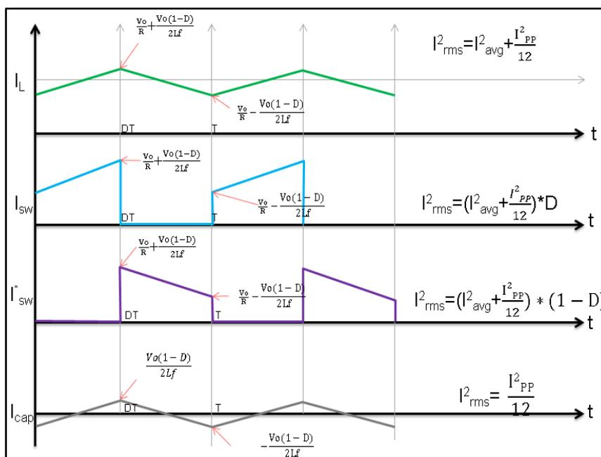
Fig(4): General Waveforms for conduction losses
